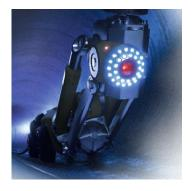
below ground. Today, sewer robots can perform many tasks from the inside. They play an increasingly important role in the maintenance of urban infrastructure. Motors from FAULHABER are used for camera control, tool functions and the wheel drive.
