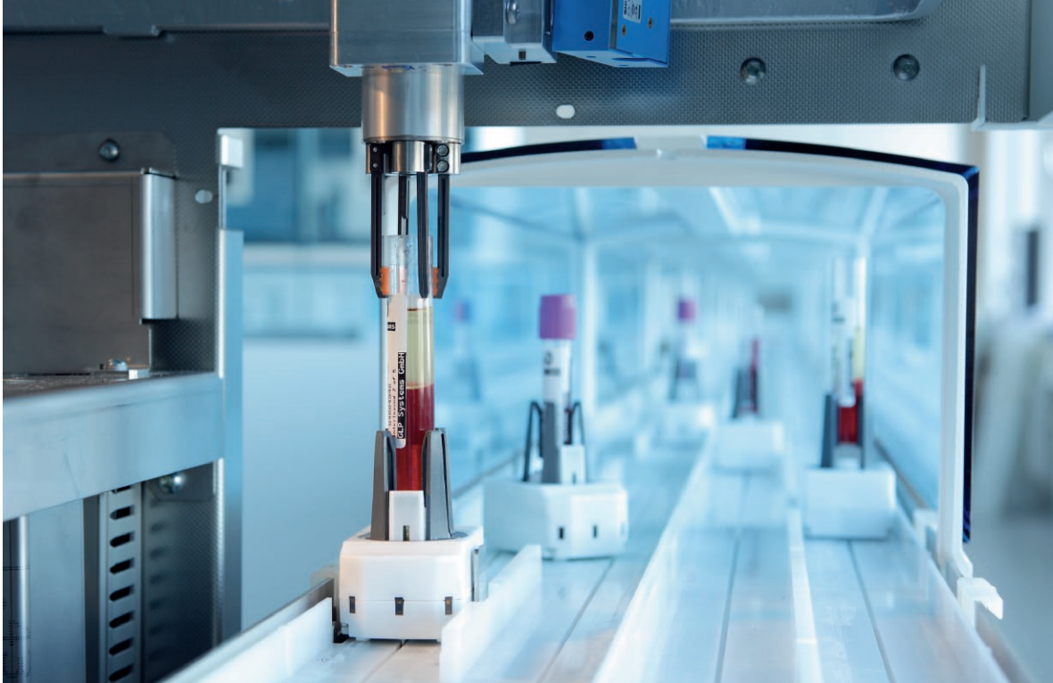
FAULHABER drives also provide movement for transporting samples between individual analysis stations.
