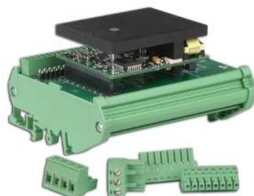
FIGURE 3.10 MC1XAZ01 and AZ_20A8 Drive Mounted on MC1XAZ01 and Phoenix Contact DIN Tray (mating connectors shown are included with MC1XAZ01, DIN tray shown for reference only, available from Phoenix Contact)
